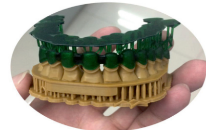
----High quality output in the shortest time. Layer: 0.025/0.035/0.05/0.1mm Speed: 8-33mm/hr, adjustable
