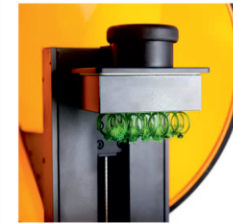
----With double-guide rail design, the forming platform runs more smoothly.
